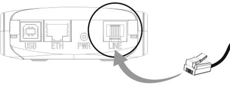
A top-down view of the SAGEM F@st modem. The ports are labeled USB, ETH, PWR, and LINE. A telephone line lead is being inserted into the LINE port, which is circled in red. An arrow points from the lead to the port. |
