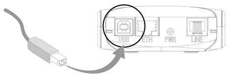
A top-down view of the SAGEM F@st modem. A USB cable is being inserted into the USB port, which is circled in red. An arrow points from the cable to the port.                                                          |
